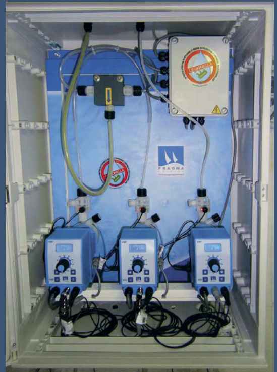
Stabilised chlorine dioxide dosing system with activator and protective film for sanitary water. All pre-assembled on an IP65 protection box with data and error communication system via Ethernet module.
